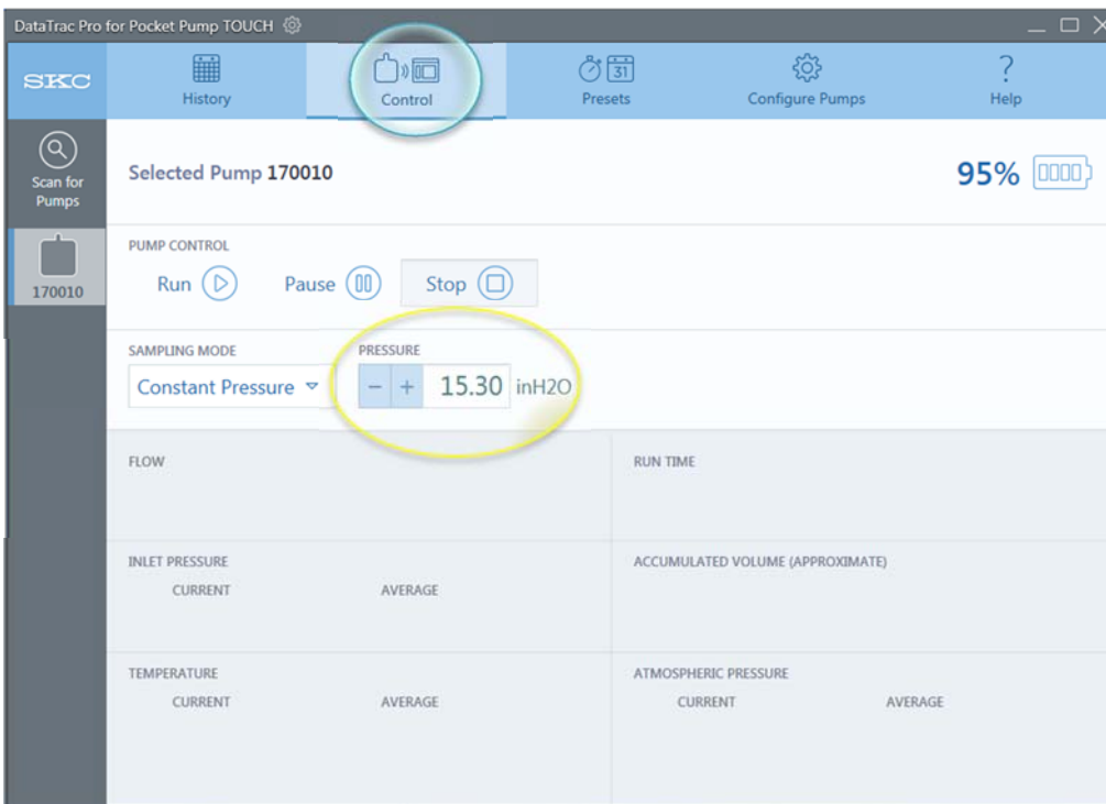
Figure 5a. Constant Pressure Mode Display Before Run is Clicked
